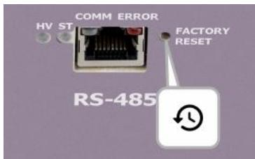
Press and hold the button, turn on the power of the meter, wait at least 3 seconds and release the button.
